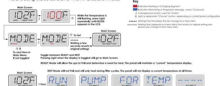
The Main Screen will display RUN PUMP FOR TEMP if the filtration pump has not run for over 1 hour. The Main Screen will display normally during Filter Cycles or when the spa is in use.
